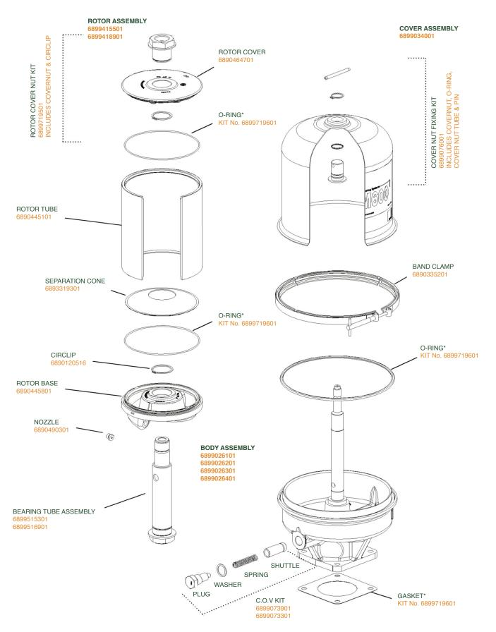
\*SEALS KIT P.N. 6899719601 COMPRISES OF: C.O.V. WASHER, FILTER BODY O RING, CVR NUT O RING, 2 x RTR BODY O RINGS & BASE GASKET
